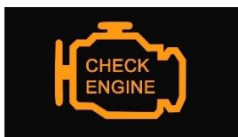
Figure 3 Example of a Malfunction Indicator Lamp (MIL)
