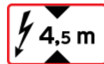
UA73: Overhead electricity lines at railroad crossing
