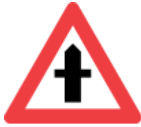
A11: Dangerous junction with a non-priority road
